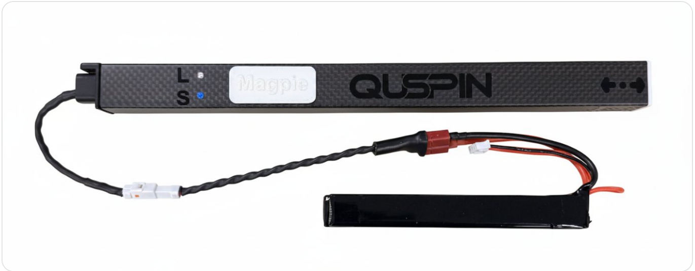
Figure 28. Magpie sled showing the logger “L” and sensor “S” LED indicators.
