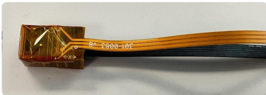
Figure 17. Fold the coil edges down and secure them with Kapton tape.
