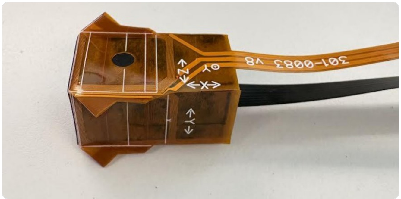
Figure 15. Align the coils with the flex-cable section on top of the sensor, then wrap them around the sensor head and rub to adhere.
